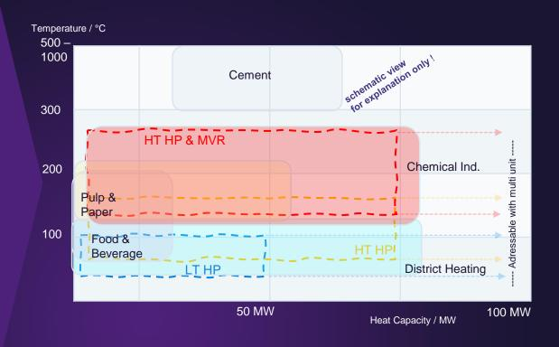
\* MVR = Mechanical Vapor Recompression; HT HP = High temperature heat pump; LT HP = Low temperature heat pump
